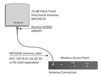
4. Locate the primary detachable antenna of the wireless device. Remove the antenna and connect the other end of the NETGEAR cable ACC-10314-01, 02, 03 or 04 to this port.
